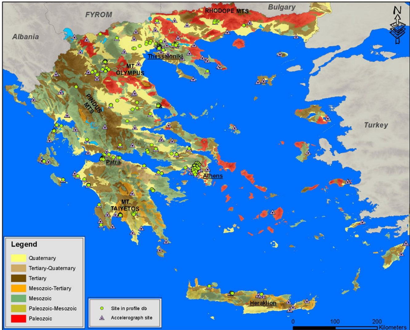
Figure 1. Geologic map of Greece showing locations of sites in profile database (PDB) and locations of strong-motion stations in site database. The geologic map used here is from digital sources (for ease of plotting) with a scale of 1:500,000. This map is for illustrative purposes only; higher-resolution maps were used to assign geologic conditions to particular sites. The color version of this figure is available only in the electronic edition.
