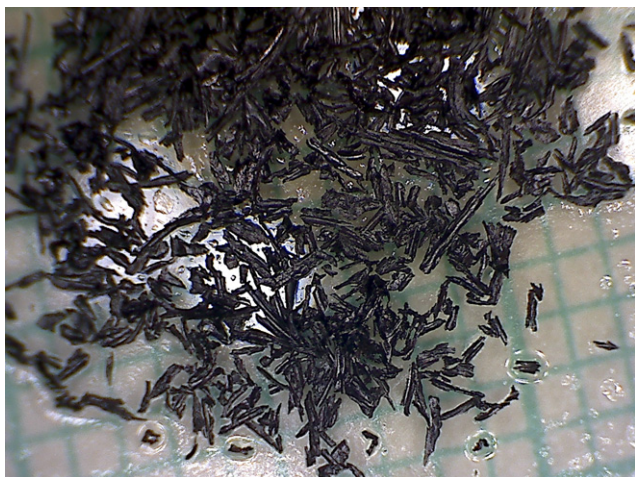
Figure 9. Photograph of U-Mo15 alloy after hydrogenation at 80 bar. The hydride consists of elongated particles 1–2 mm long displayed on a background of a millimeter grid.
