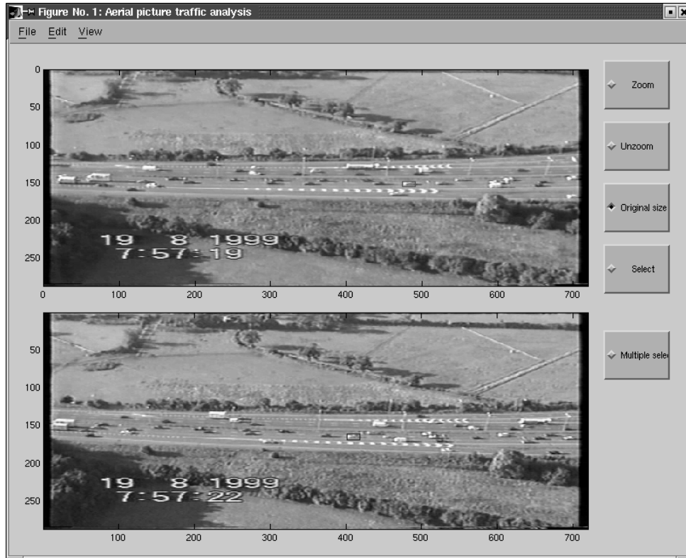
Figure 6: Screen capture from our automatic image analysis software package. The operator has selected a vehicle, top picture approximate coordinates (490,150) and the software has automatically tracked the vehicle for 3 seconds (bottom picture).
