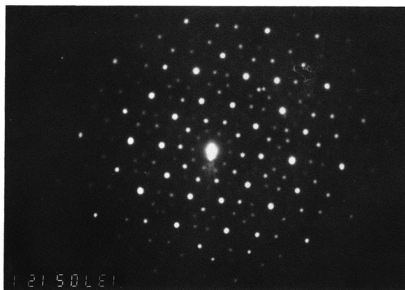
FIGURE 14. Electron diffraction pattern by the author of a quasi-crystal of Mg_{32}(Al, Zn)_{49} .
