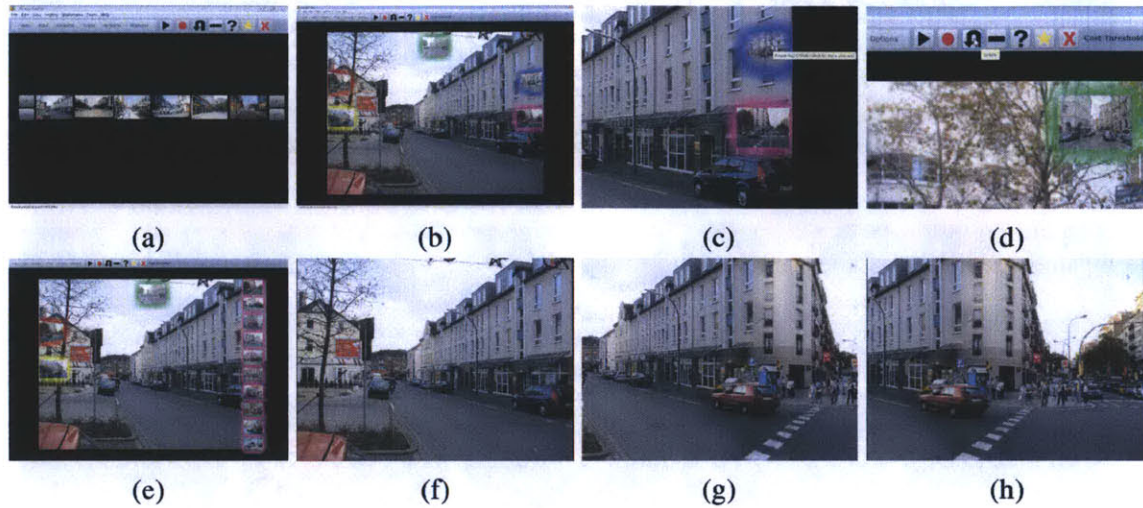
Figure 7.18: A screen shot of the interactive system. (a) Selecting an image to start browsing. (b) The current image is shown in the center and the next image for each motion (forward, rotate left/right, translate left/right) is shown as an inset. (c) Selecting rotate right motion. (d) The user can undo the current transition. (e) The next image for a particular motion (here move right) can be also interactively chosen from the top 10 matching images displayed on the side. (f-h) show the first, middle, and last frame of a rotate right motion sequence.
