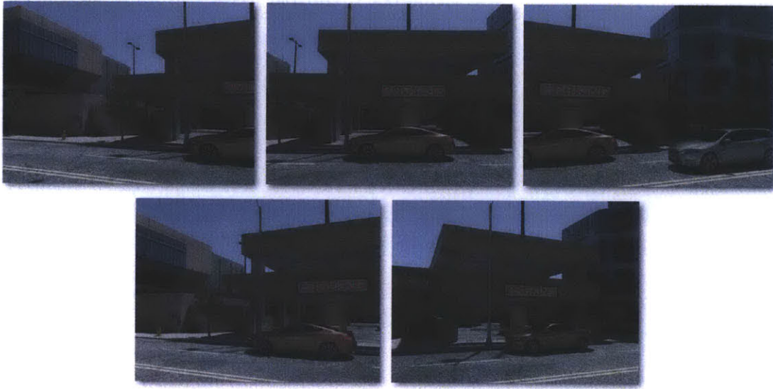
Figure 3.4: Samples images from the virtual city. Top row: Scene from a panning camera at 22.5 degree rotation stops. Bottom row: Images taken from a different camera viewpoint and location of the center image in the Top row .
