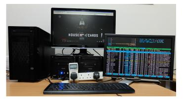
Fig. 1: Our video playback testbed. The black Shuttle systems (centre) were used for the playback experiments, and are connected to the Kill-A-Watt/MoteWatt power meter (centre-left, just above the keyboard). The mini-tower on the left is the experiment-controller, not part of the system being measured. The energy consumption of the display units was not measured: one shows the video being played back (centre), the other shows part of the measurement system (right).
