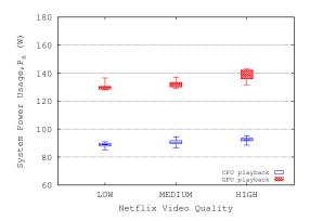
Fig. 5: System wide power usage for video playback using a CPU vs using a GPU. The GPU adds considerable idle power to the system, but does not offer any gains in efficiency.
