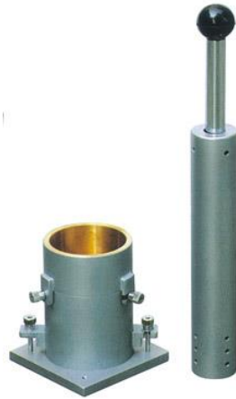
Figure 12: Soil Compacter (Standard Compaction Test)
