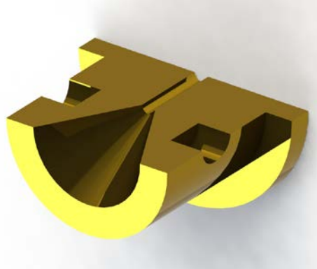
Figure 19: Section view of a SolidWorks rendering of the die
