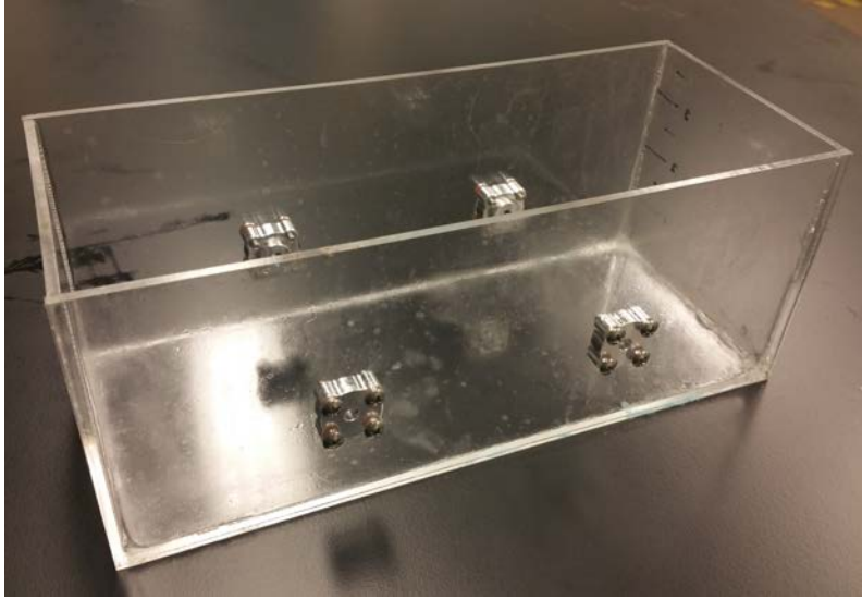
Figure 20: Acrylic trough to hold cooling fluid
