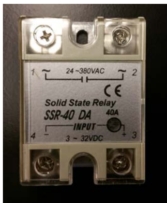
Figure 23: Fotek solid-state relay for switching high voltage and high current
