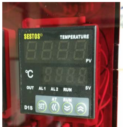
Figure 22: Sestos DIS-VR-220 PID temperature control unit
