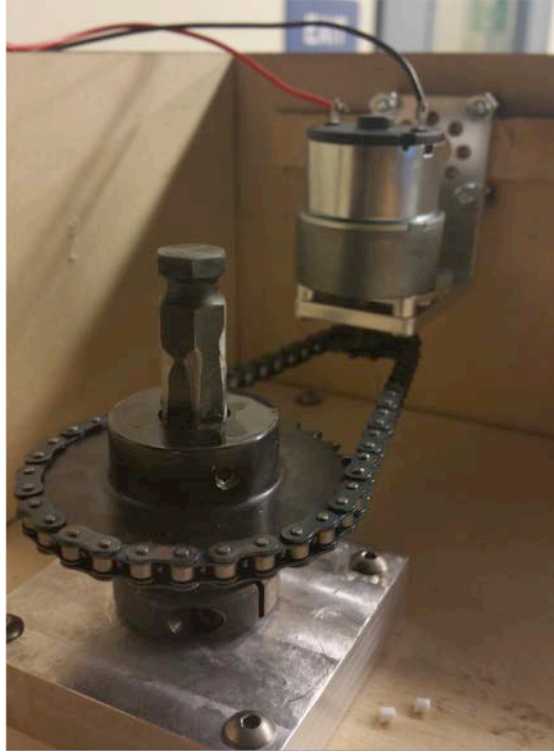
Figure 24: Chain drive connecting motor and auger
