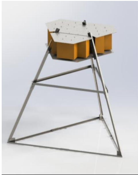
Fig. 6: Second derrick design, assembly process was not approved.
