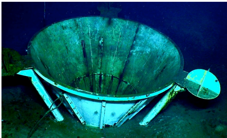
Fig. 2: Existig borehole with tilted and damaged reentry cone. Source: http://www.mstfoundation.org/story/DEBI-SELECT
