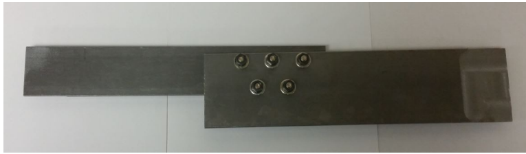
Fig. 13: Bolt test assembly used in this experiment.
