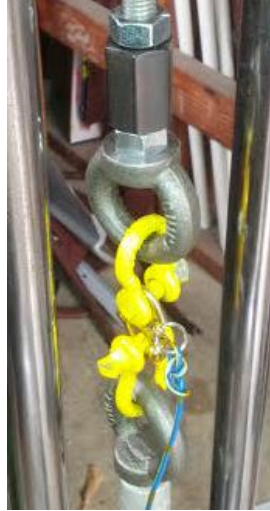
Figure 3.3-4: Quick release mechanism as installed
