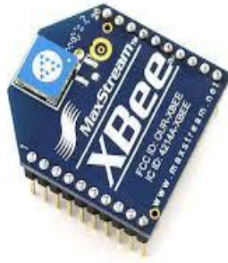
Figure 3.1.4.1-1: The XBee radio transmitter and receiver module.
