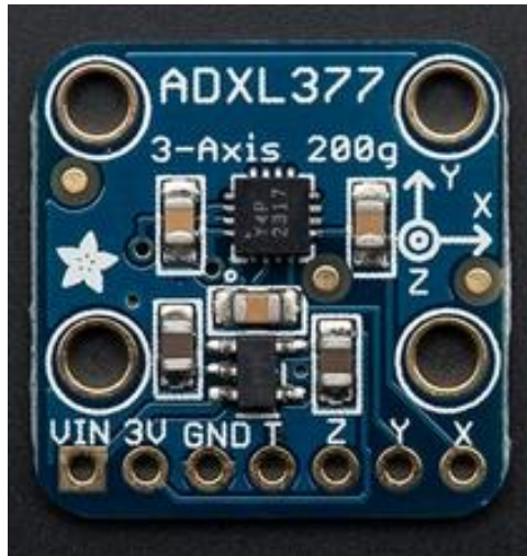
Figure 3.1.4.2-1: The ADXL377 accelerometer integrated into a prototyping break-out board.
