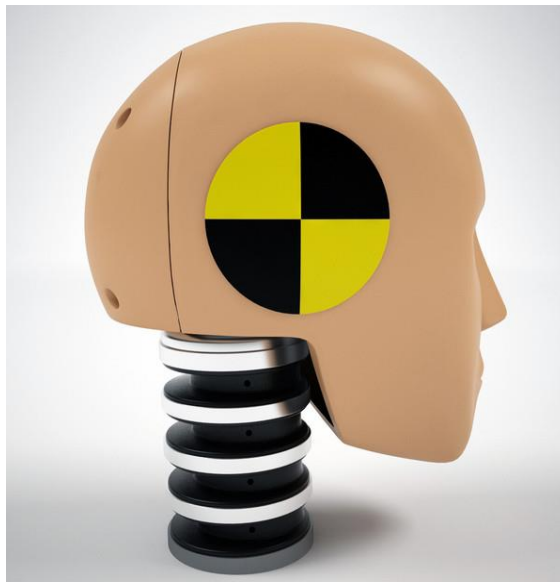
Figure 3.4-1: Hybrid III commercial crash test dummy head and neck assembly.
