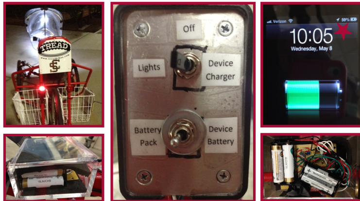
Figure 5.2 Top Left: vehicle lights. Bottom Left: circuit housing. Center: user interface box. Top Right: iPhone being charged by vehicle. Bottom Right: removable batteries
