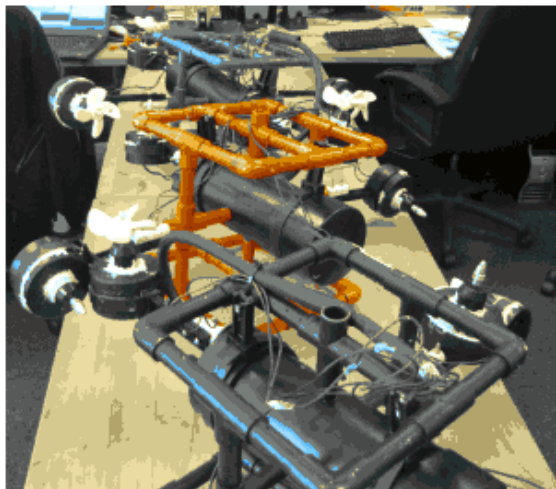
Figure 27: 3 Constructed PVCROV 's
