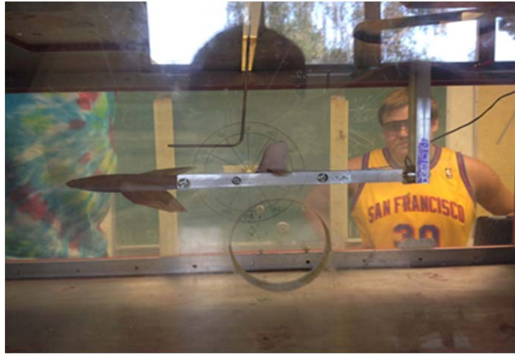
Figure 16: Testing of 12.5 degree wing sweep
