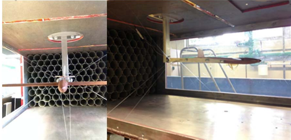
Figure 18: Non-elastic wire used to secure sting
