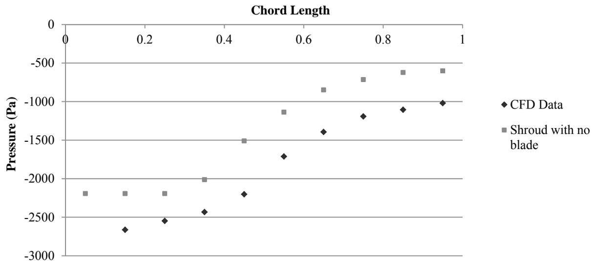
Figure 25: Pressure values along the shroud for CFD and physical testing
