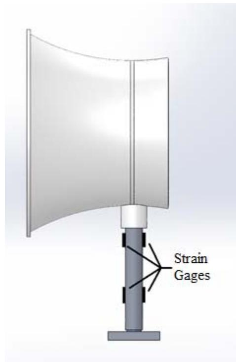
Figure 24: Location of strain gage sensors on the shroud post
