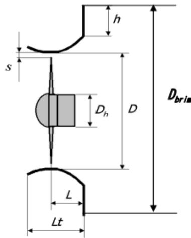
Figure 6: Schematic of wind-lens turbine [8]
