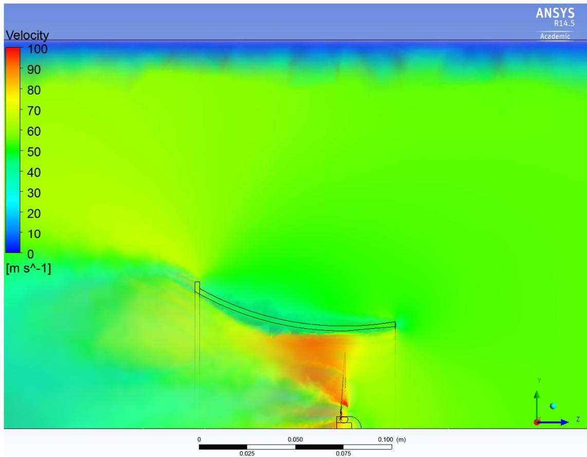
Figure 22: Volume rendering of wind velocity as air flows past a spinning blade.
