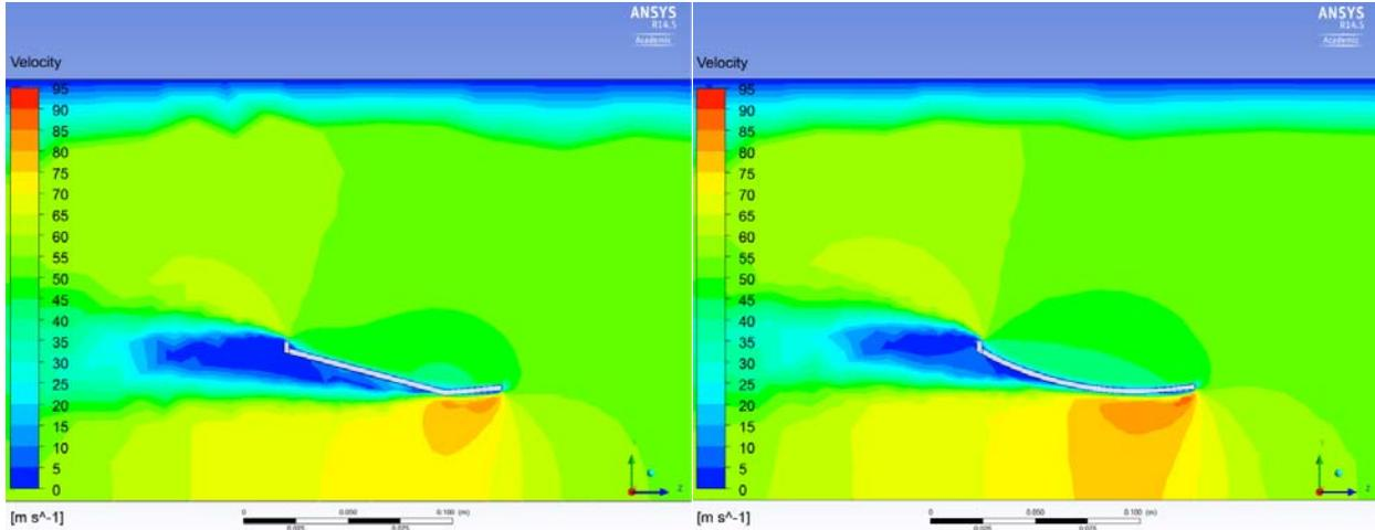
Figure 13: Cross sectional view of a quarter shroud geometry showing wind velocity contours around shroud without curvature (left), and with curvature (right)
