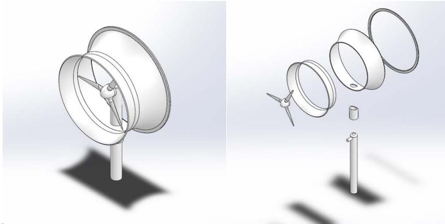
Figure 8: Sketch of assembled shroud (left) and exploded view of shroud system (right).
