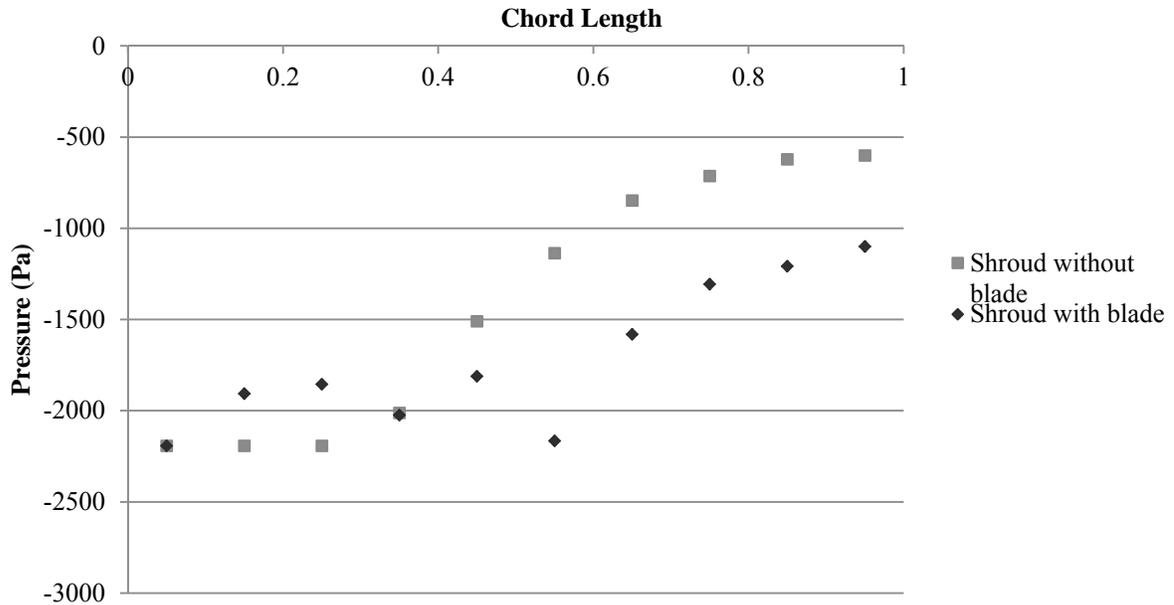
Figure 26: Pressure values along shroud with and without rotating turbine
