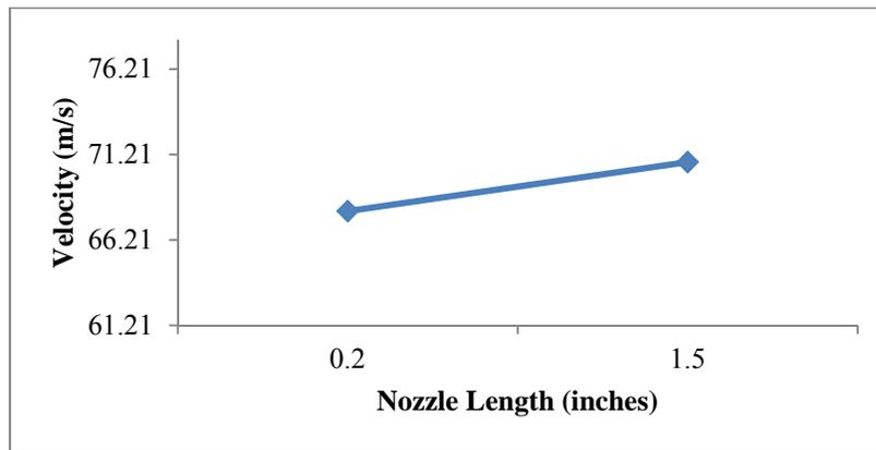
Figure 17: Effect of the nozzle length on the average velocity.
