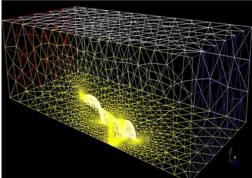
Figure 11: Tetrahedron mesh used to model a quarter of the shroud geometry.
