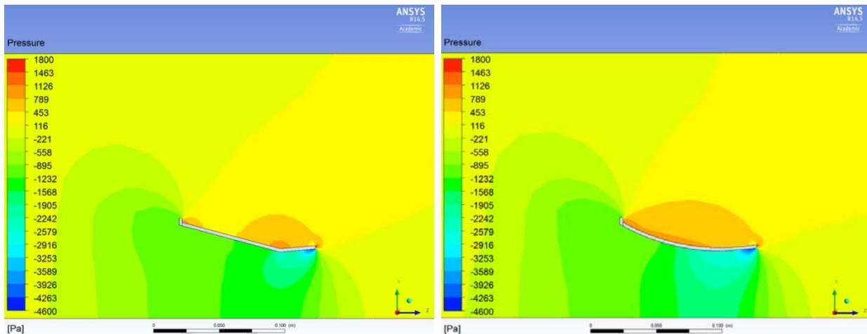
Figure 12: Cross sectional view of a quarter shroud geometry showing pressure contours around shroud without curvature (left), and with curvature (right)
