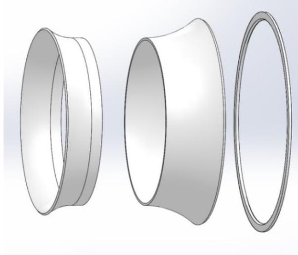
Figure 10: Exploded view of shroud components: diffuser (left), nozzle (center) and flange (right).
