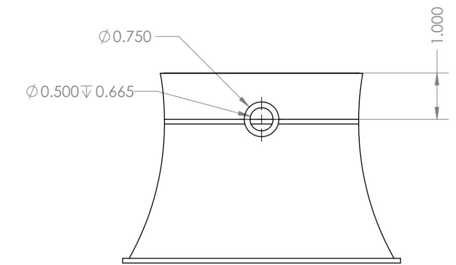
**INNER CURVATURE DETAIL DIMENSIONS FOR SECTION A-A**
