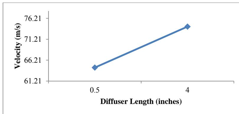
Figure 18: Effect of the diffuser length on the average velocity.
