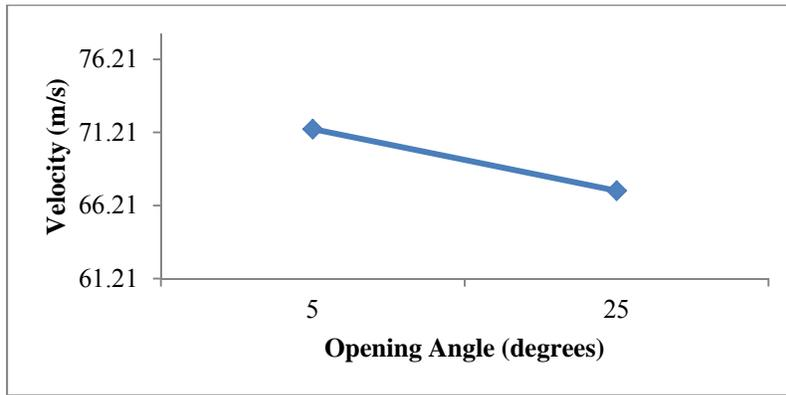
Figure 16: Effect of the opening angle on the average velocity.
