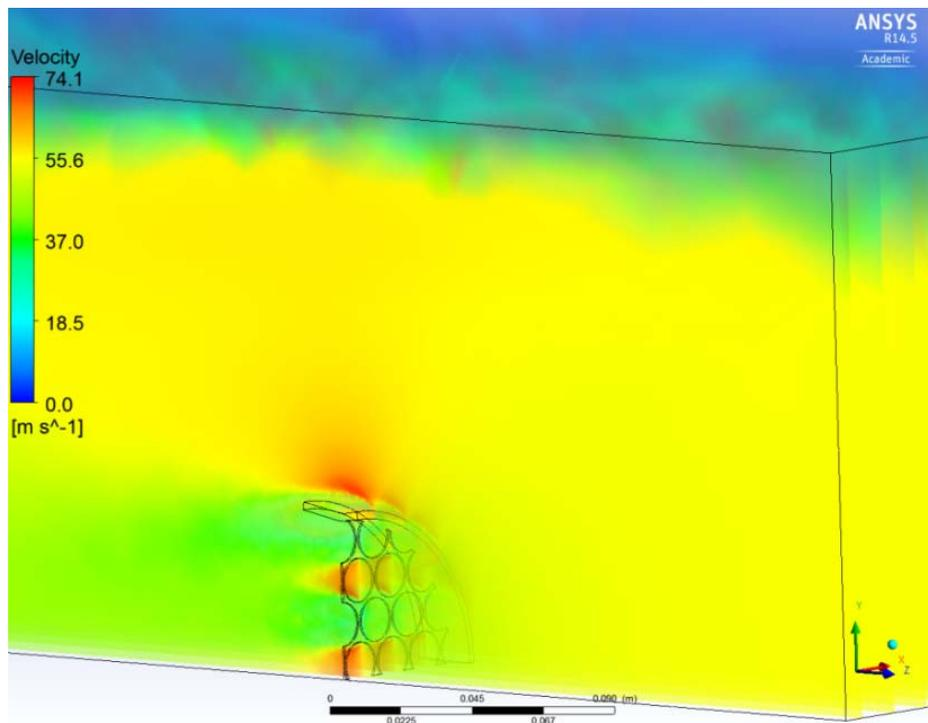
Figure 21: Attempt to model turbine as perforated screen
