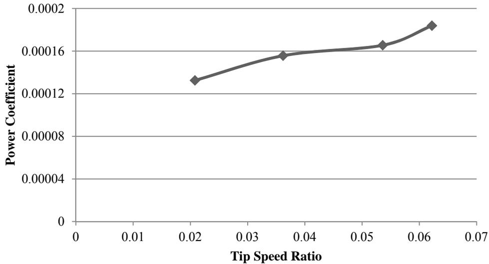
Figure 27: Power coefficient based on the tip speed ratio of the turbine blade.
