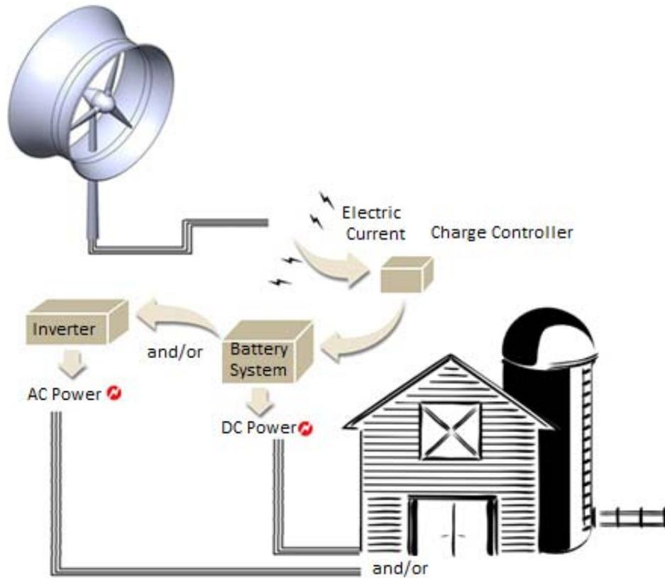
Figure 7: System level sketch of shrouded small wind turbine.
