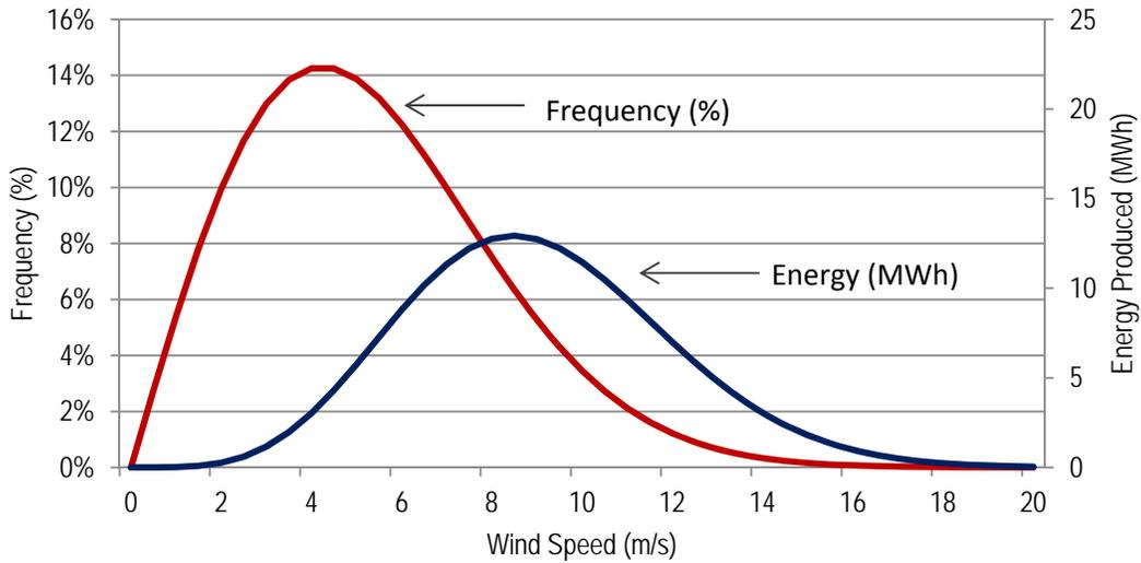
Figure 3: Frequency and energy yield of wind speeds [5]
