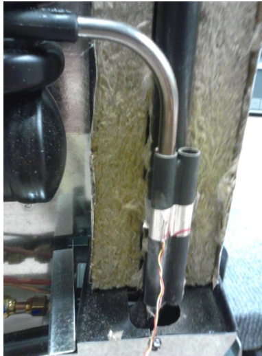
Figure 3.2: Boiler Column with Electric Heater
