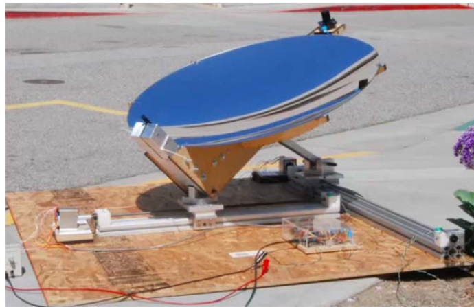
Figure 3.6 – Implementation of original Solar Tracker without receiver module (Barker et. al)
