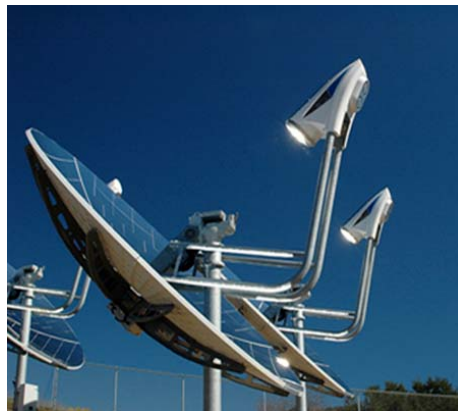
Figure 2.8: Infinia CSP system using the Stirling Engine
