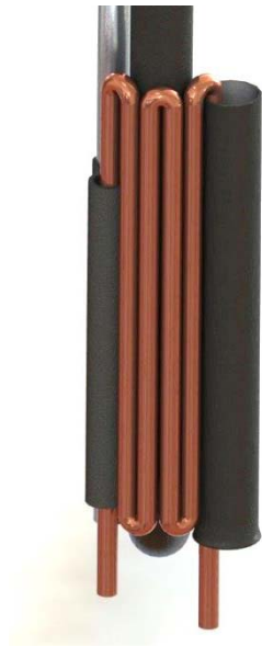
Figure 3.3: Proposed design and orientation of heat exchanger in SolidWorks
