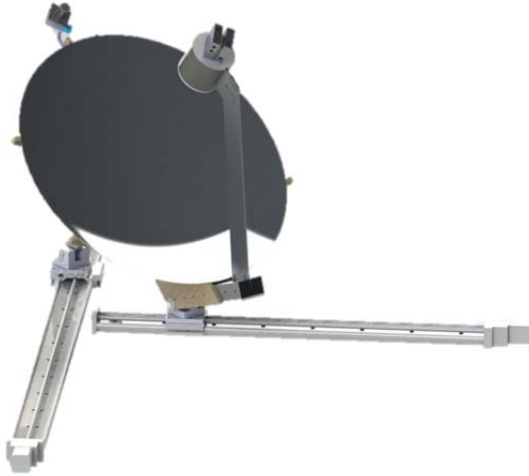
Figure A10-2: The parabolic mirror is supported and moved by two separate tracks which are computer controlled. This ensures the mirror stays at an angle normal to the sun so that the energy produced is maximized.
