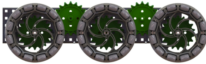
Figure I.5: Solidworks rendering of a side view of the drive train.
