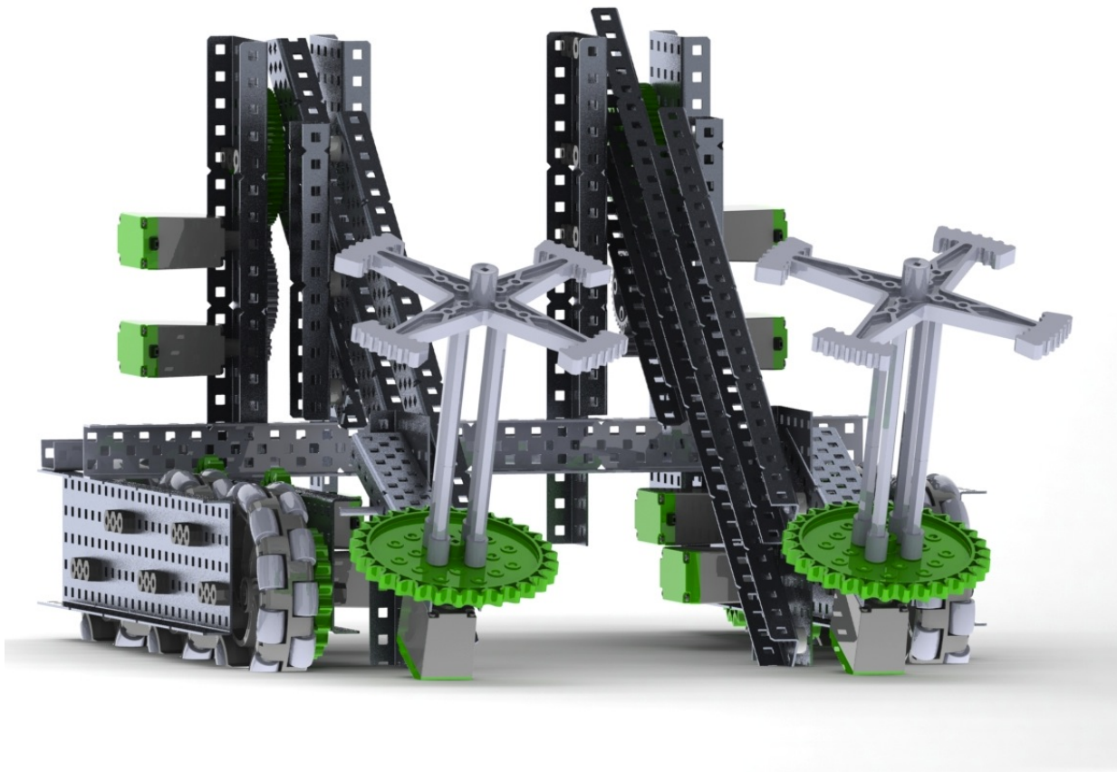
Figure I.1: Solidworks rendering of the front side of the robot.
