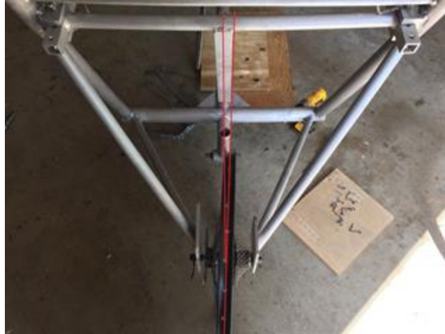
Figure 3.6.2 Misalignment of the rear wheel due to axle warping. The wheel was pointing about 3 degrees off center as shown by the red lines. The line on the right shows the original direction of the wheel and the left shows the direction the wheel needed to point.
