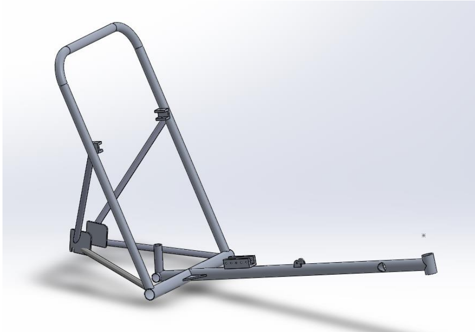
Figure 3.1.2.2 CAD rendering of the main vehicle frame
