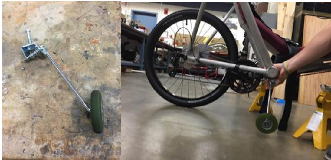
Figure 3.6.4 Balance wheel design (left) and expected placement(right). The wheel is only shown on one side but after tests are done on wheel strength, another wheel will be added to the other side to prevent over adjustment and tip over.
