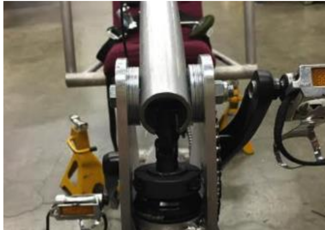
Figure 3.2.3.4 Housing tube and u-joint connection
