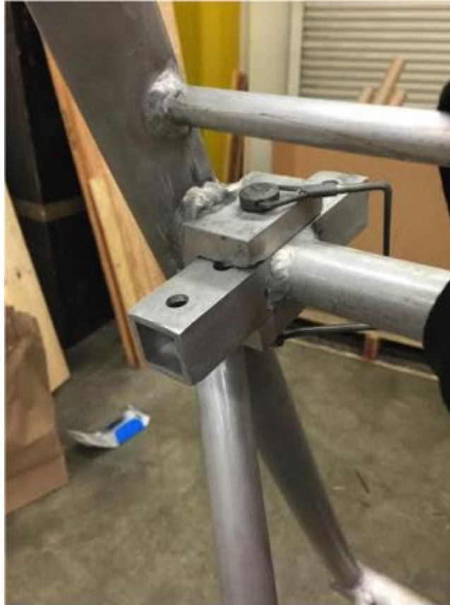
Figure 3.2.3.2 Pinned right seating bracket
