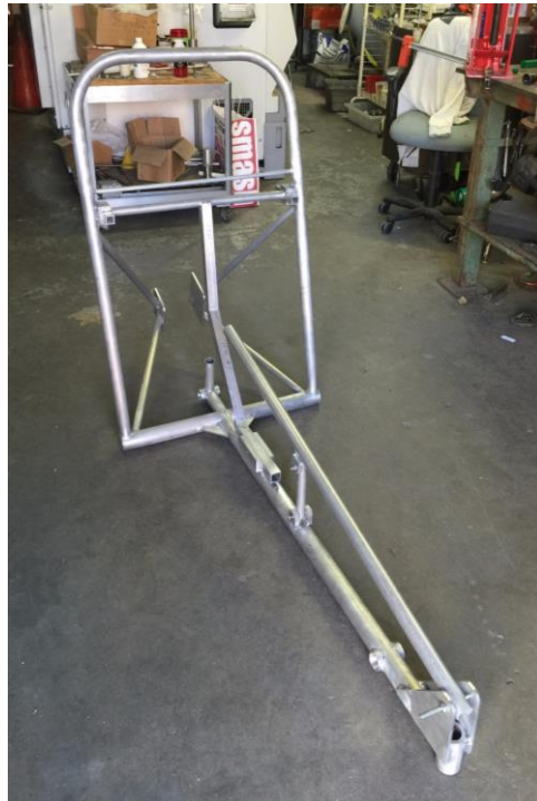
Figure 3.1.4.1 Fully welded frame from Chavez Welding
