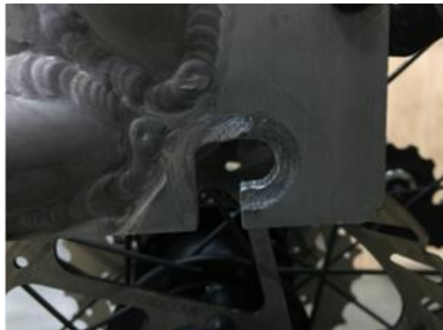
Figure 3.6.3 The rear axle mount was filed backwards 1/2 in. This allowed the rear wheel to point in the same direction as the rest of the bike.
