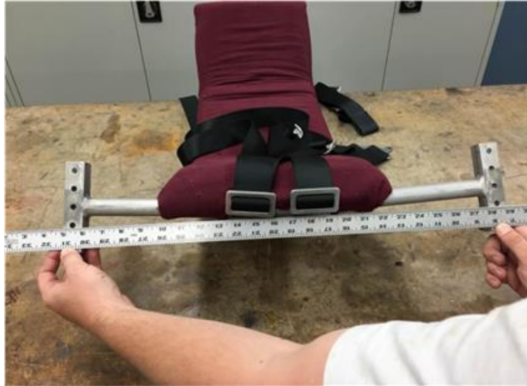
Figure 3.6.1 Bending of Seat Frame after heating treating. The bend prevented full adjustability in the seat. For the rest of testing and assembly the seat was fixed in its middle position.
