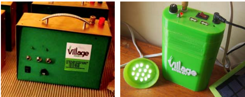
Figure 3: On left, Village Energy sheet metal solar lantern enclosure. On the right is solar lantern enclosure improved aesthetics from 3D printing.
