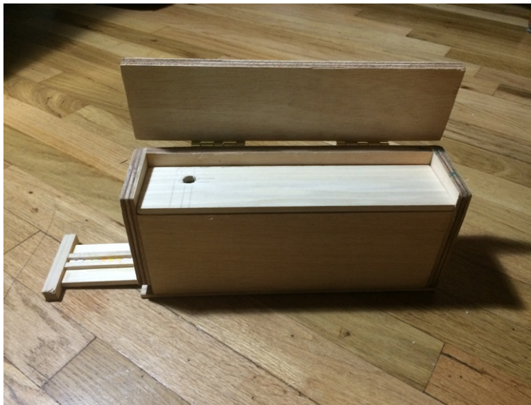
Figure 2: Hardware prototype 1 exterior with open lid, closed cover, and partially removed test strip slide
