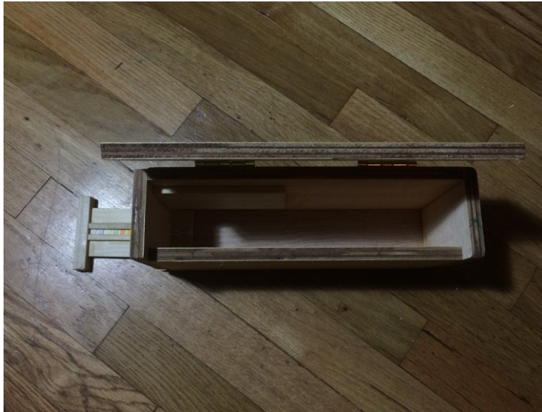
Figure 3: Hardware prototype 1 interior with open lid, removed cover, and partially removed test strip slide
