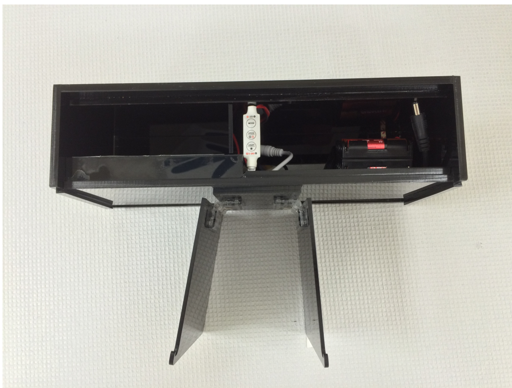
Figure 5: Hardware prototype 2 interior view. As seen from left to right: downward-facing LED strip panel, dimmer switch, power supply.
