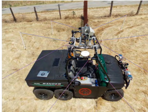
Figure 10.6: The resulting web from attaching string to each camera and then tying those strings to posts and placing them in the ground when the post left the field of view of the respective camera.
