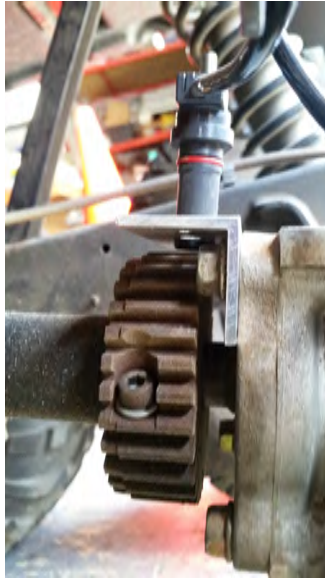
Figure 8.2: Hall Effect Tachometer
