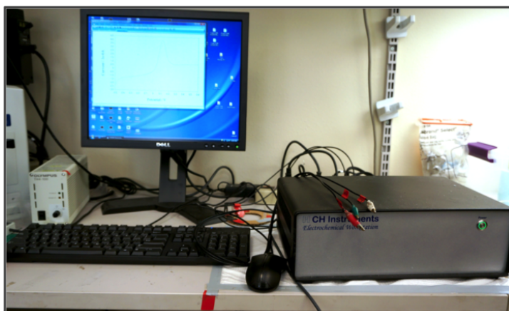
Figure 1.2: The CH Instruments 730D Electrochemical Analyzer
