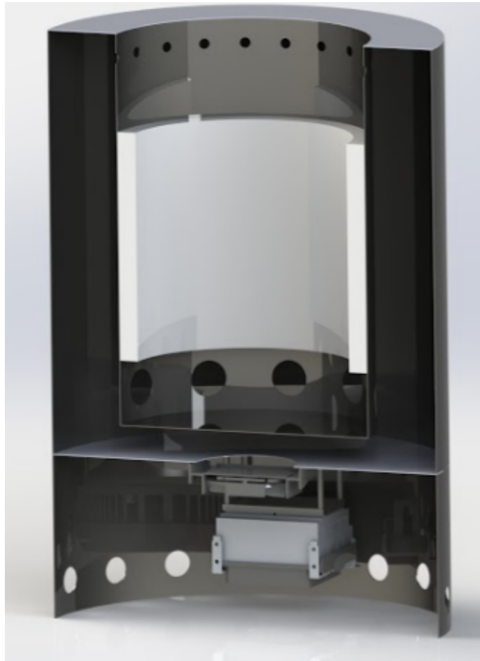
Figure 3.1: Overview of Combustion Chamber
