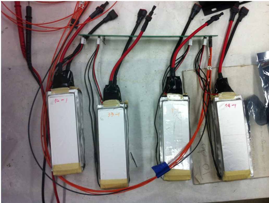
Figure 9: Four modules connected to a single PCB.
