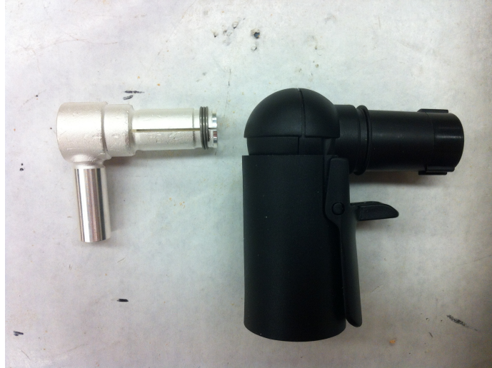
Figure 49: High voltage connectors to connect high voltage wire to motor controller from either the battery pack or motor. Connector is shown to the left, with the plastic protective casing shown to the right of it.
