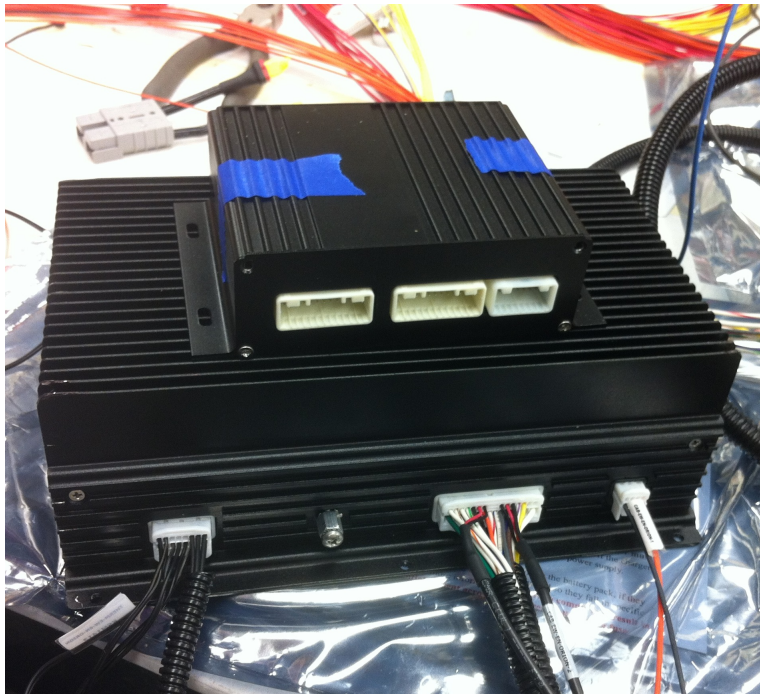
Figure 12: Photograph of the Orion BMS system.
