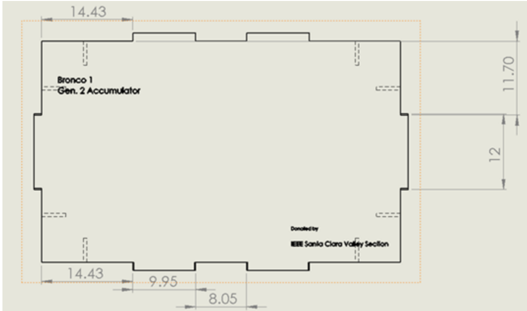
Figure 16: Part drawing of the battery pack front panel with tabs.
