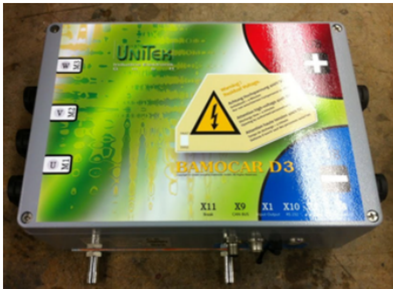
Figure 44: Unitek Bamocar D3 series motor controller. Water inlet and outlet nozzles for liquid cooling can be seen on bottom of controller.
