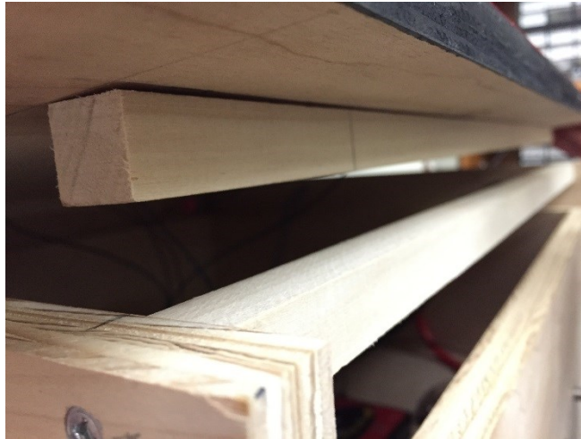
Figure 3.6: Docking station platform alignment bars
