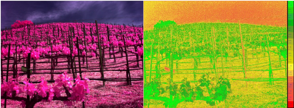
Figure 1.2: Example of a raw multispectral image and its processed counterpart. Green indicates vegetation in good health, yellow indicates moderate health, and red indicates poor health or areas of non-vegetation.
