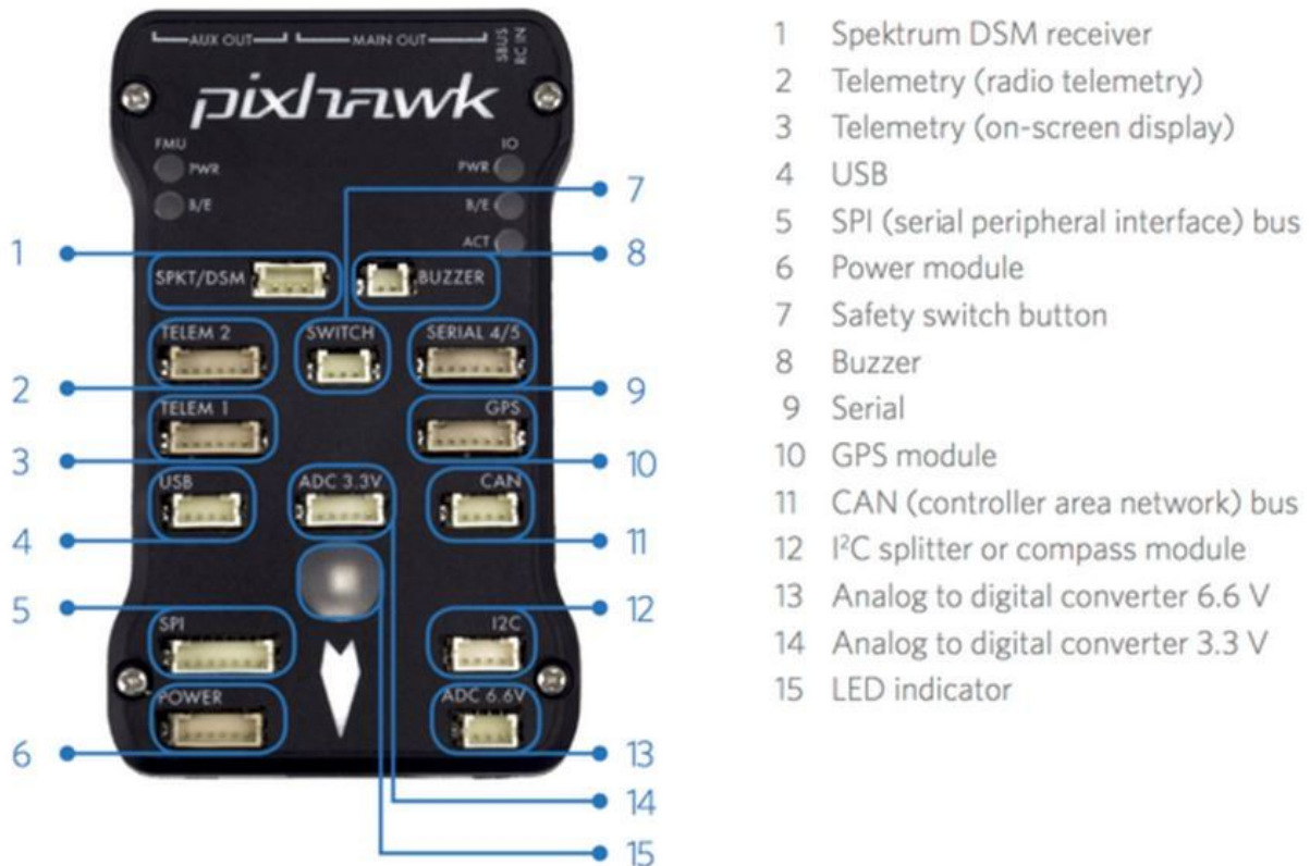
Figure 19: Layout of the 3DR PixHawk autopilot system and the key connections [12].
