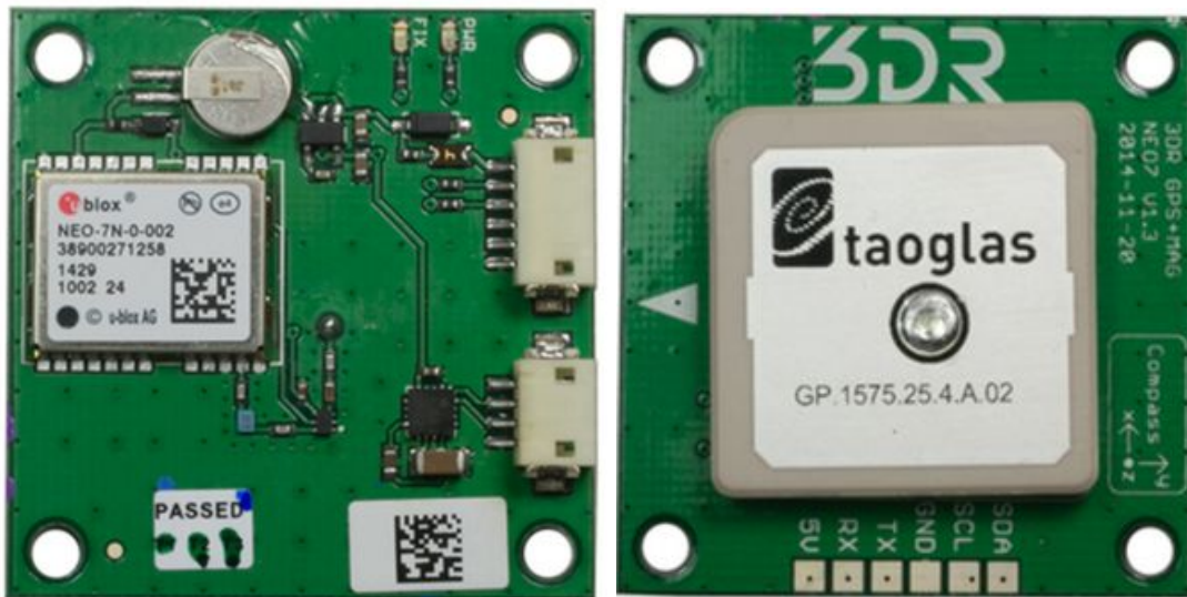
Figure 20: U-Blox GPS NEO-7N (Left) & Honeywell HMC5883L Digital Compass (Right) [22]
