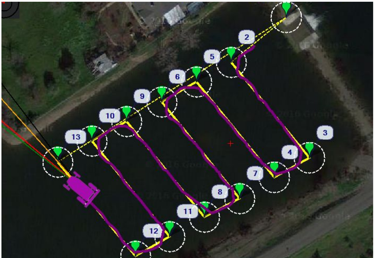
Figure 35: Screenshot of predetermined lawn mowing path and actual route during mission. (A video of this run can be found at https://www.youtube.com/watch?v=oFY5hq9z18o )
