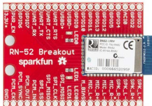
Figure 3.5 - Microchip Technology RN-52 (reproduced without permission)
