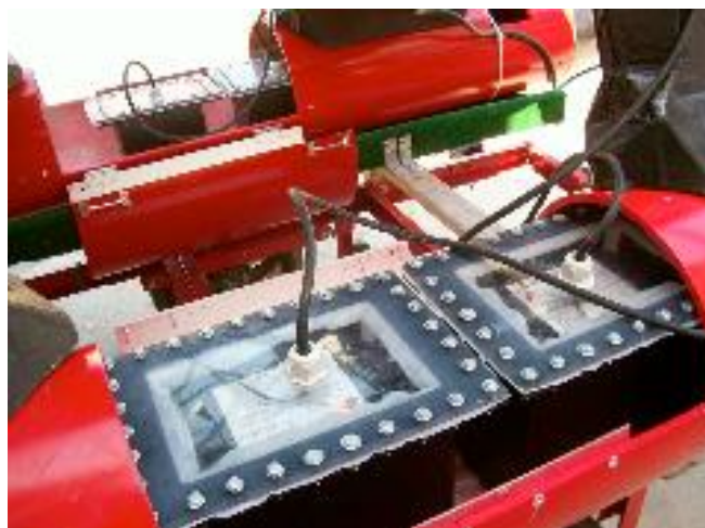
Figure 2.5: Batteries mounted in water tight containers placed in the hull of SWATH[39]
