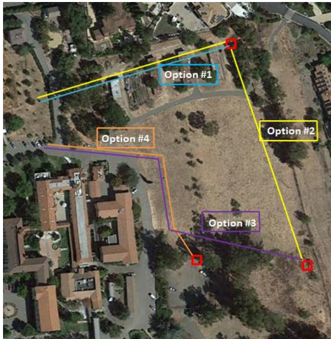
Figure 9 - Piping network options
