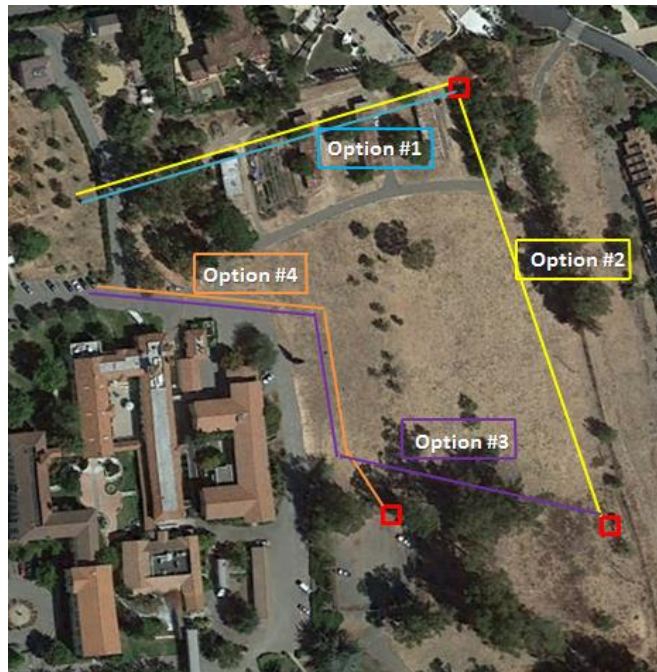
Figure 30 - Piping network options
