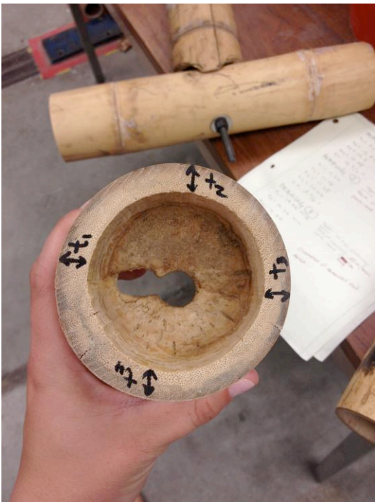
Fig. 5. Test specimen and node fibers before node crushing.
