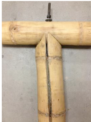
Fig. 1: Anchor bolt connection of the brace frame
