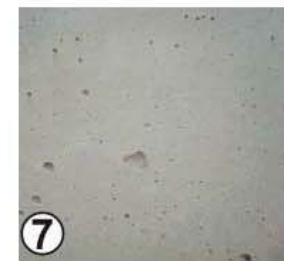
⑦ Raised Planters and Post Bases: exposed poured-in-place concrete (planters may be Trex or an alternative material)
