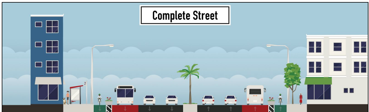
Figure 6. Bus-only lane with protected bike-lanes that is integrated into the sidewalks
