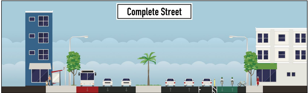
Figure 7. Complete Street example with bus lane-only and bike route on one side of the street
