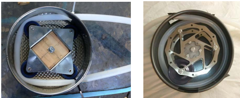
Figure 2.2 Low Cost Home-built Peristaltic Pumps
