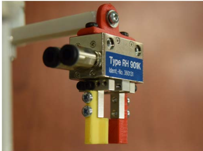
Figure 2.2: 3-D gripper “fingers” and rotational top joint created in Solidworks™
