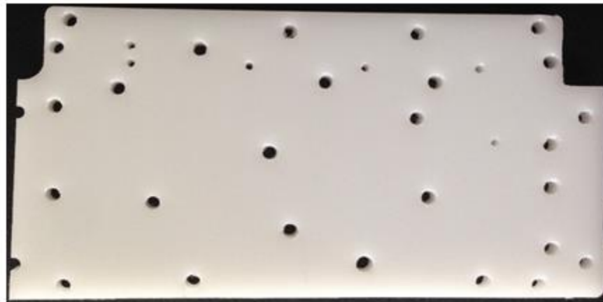
Figure 8. Prototype 2 made out of high density polyethylene (HDPE). The perimeter of HDPE back plate has incomplete screw holes. Prototype was made with a laser cutting machine with a tolerance of 0.001". Incomplete screw holes is due a lack of HDPE resulting in a smaller width than desired.
