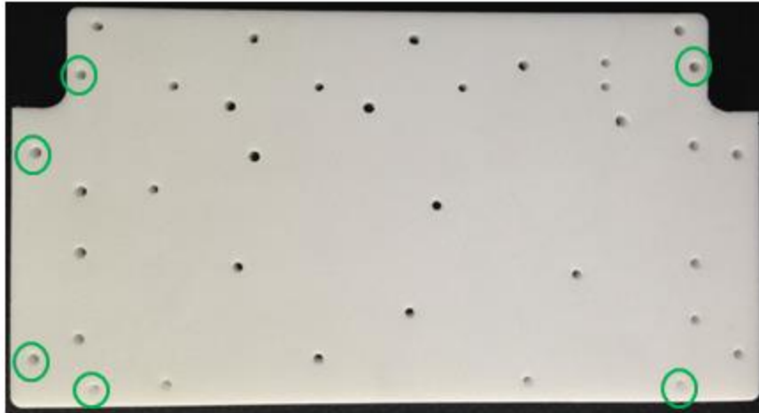
Appendix G. Prototype 3 made out of PTFE. Figure demonstrates all complete screw holes in green (those screw holes that were incomplete in prototypes 1 and 2).
