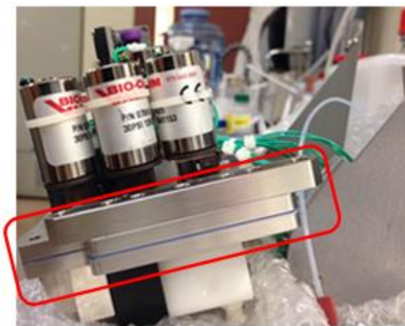
Figure 5. Internal components of MicroCal ITC200 washing module. Image of the internals of the washing module illustrating the original hydraulic manifold outlined in red.
