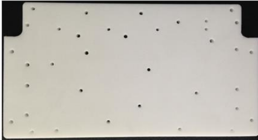
Figure 9. Prototype 3 made out of polytetrafluoroethylene (PTFE, Teflon). This prototype shows successful fabrication without openings in the screw holes along the perimeter.
