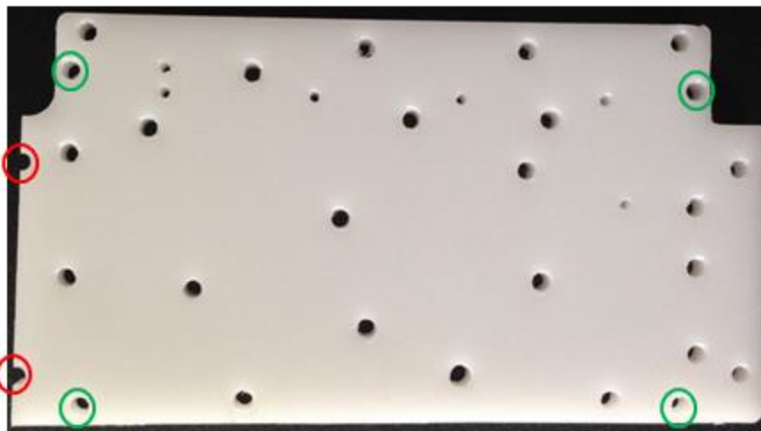
Appendix F.. Prototype 2 made out of HDPE. Contains the incomplete structural screw holes in red and the corrected structural screw holes in green. The corrected screw holes are the holes that were incomplete in Prototype 1.
