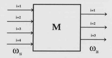
With multiple inputs and outputs the mass balance equations are as follows (subscripts indicate mass balance of each flowing substance):
