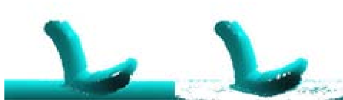
Figure 1. Using RANSAC, background surface was detected and removed.
