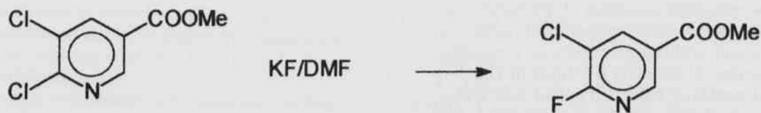
Fig. 1. Nucleophilic displacement of chloride by fluoride at 158°C
