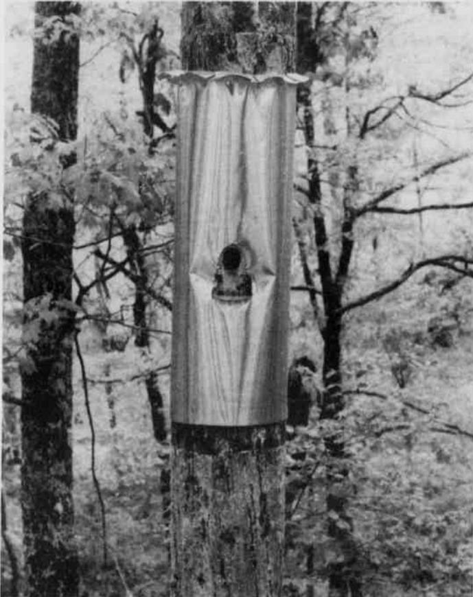
Fig. 3. Single-strip Squirrel Excluder Device (SQED) with sap-deflector on the Ouachita National Forest, Scott County, Arkansas. (Cluster 1257/20 - Tree #13).
