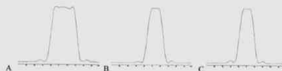
Fig. 7. Profiles obtained using the unmodified PRESS sequence. A. Profile in the x direction using a 90^\circ pulse. B. Profile in the y direction from a 180^\circ pulse. C. Profile in the z direction.
