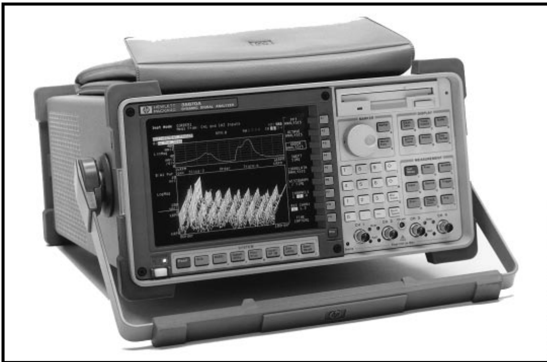
FIGURE 16 HP 35670A Digital Signal Analyzer (37)
