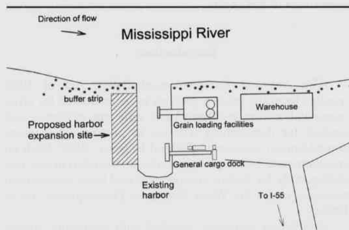
Fig. 1. Diagram of New Madrid County existing harbor and proposed widening site. Asterisks indicate areas with mature trees.
