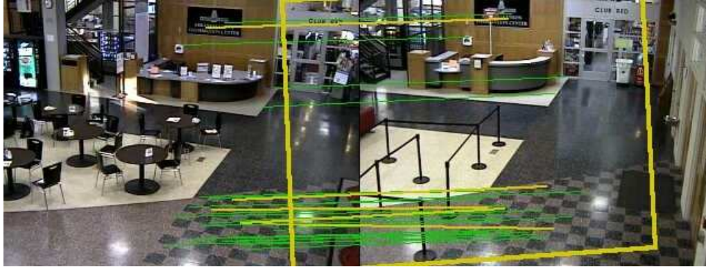
Figure 37 - Input1 (left) to Input2 (right) matched using features with counts 0-5 (Input1) and 0-10 (Input2). Matches drawn in green (correct) and yellow (wrong) [16]
