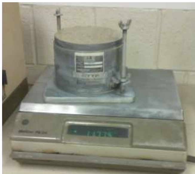
Figure 3.37. Weight measurement of base and mold containing compacted base course sample.
