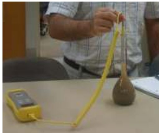
Figure 3.34. Temperature measured of soil sample de-aired water solution in pycnometer as measured using a digital thermometer.
