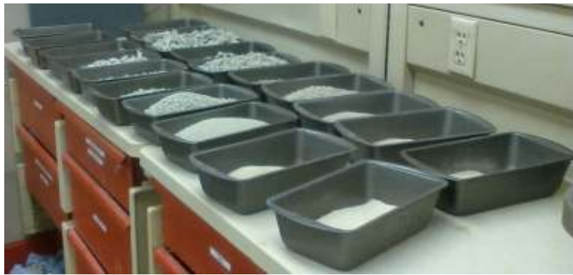
Figure 3.35. Individual grain sizes are placed in separate metal pans after sieving.
