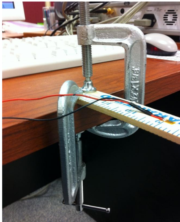
Figure 50 – C clamps holding the beam to the desk. This ensures that the beam has a rigid anchor point allowing for the cantilever beam equations to be used.
