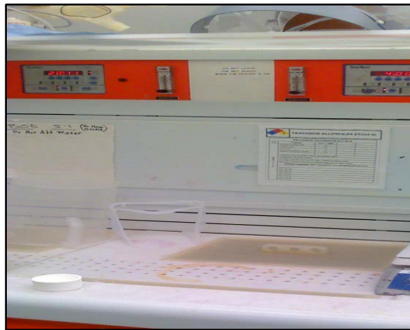
Figure 3.7. This wet bench stored the Transene type D solution for Al etching [49].
