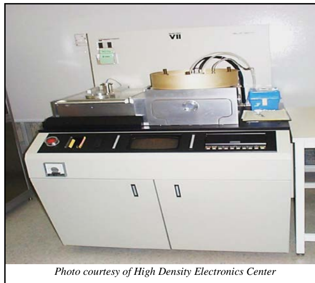
Figure 3.4. The PECVD system used in the deposition of a-Si films [49].
