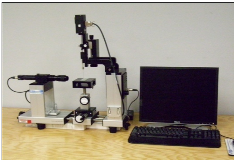
Figure 3.11. The contact angle machine features an in-line camera and power syringe system which dispensed droplets for water and oil CA testing [49].
