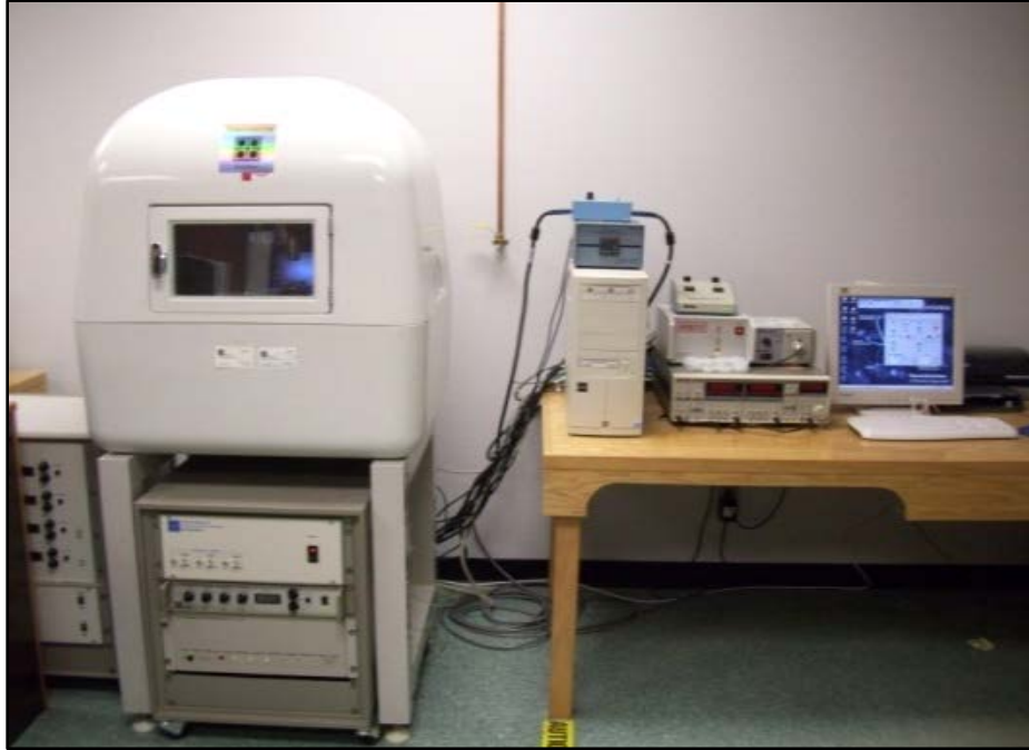
Figure 3.12. The Hysitron TriboIndenter was used in the friction testing of samples.
