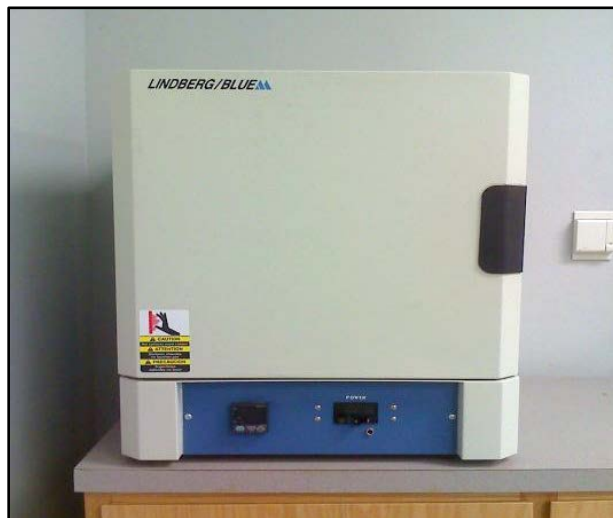
Figure 3.6. The furnace shown here was used to anneal the samples for nano-texture creation [49].
