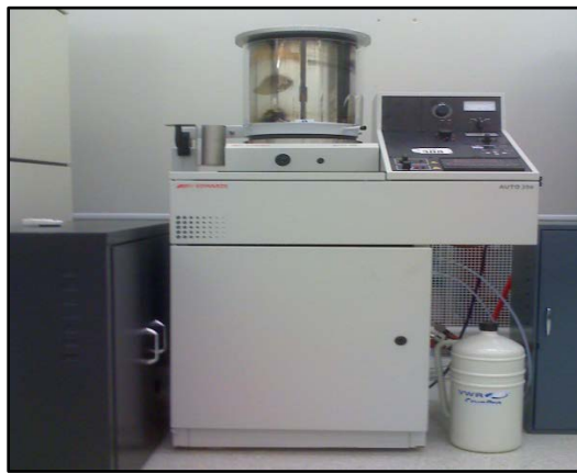
Figure 3.5. The Edwards thermal evaporator was used for the deposition of Al onto the Cu/a-Si substrates [49].
