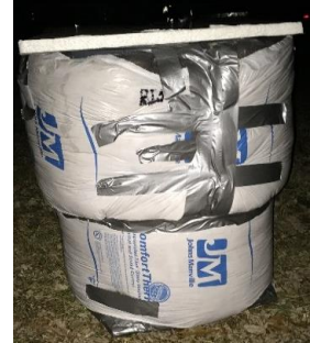
Figure 4: Insulated water reservoir.
