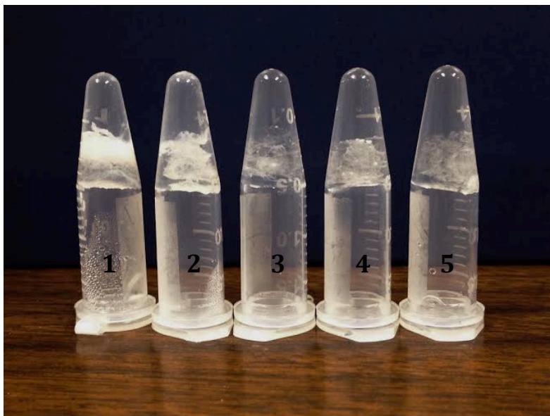
Figure 6: Hydrogel Samples at Extreme Temperatures. Immersion temperatures decrease from left to right. Sample 1 was immersed in 70C, sample 2 was immersed in 55C, sample 3 was in 37C, sample 4 was in 27C, and sample 5 was in 4C.
