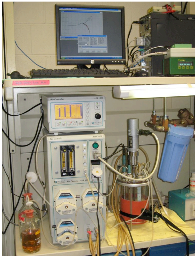
Figure 2: Set up of the bioreactor and monitoring equipment used for fed-batch fermentation of E. coli [5]
