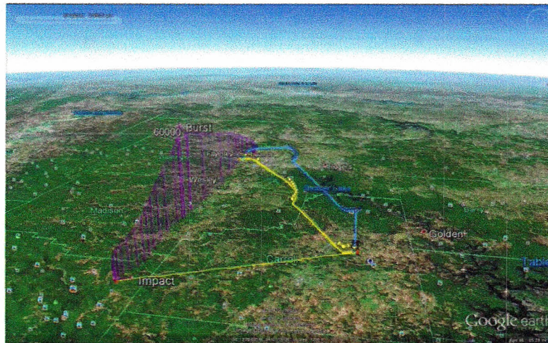
Figure 4. Predicted flight path shown in purple, actual tracking results shown in blue, ground track shown in bolded yellow, straight-line distance between predicted and actual landing point in thin yellow.
