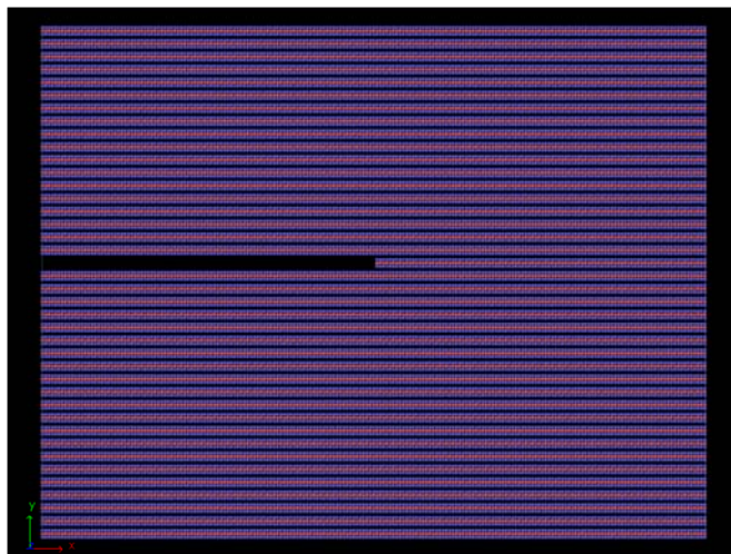
Figure 17. The image above shows the deletion of a half plane of MoS 2 and the resulting void caused by this deletion.
